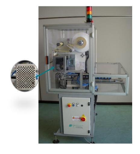
To meet logistical labelling needs, Label Engineering offers Apply Code 128, suitable for the application of self-adhesive labels on one or two adjacent sides of pallets, according to specific industry standards including GS1, ODETTE, VDA 4902, AIAG, MAT.
