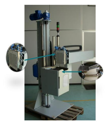
APPLY CODE A4, specific for the application of A4-size self-adhesive labels on one or two adjacent sides of pallets, according to specific industry standards.
