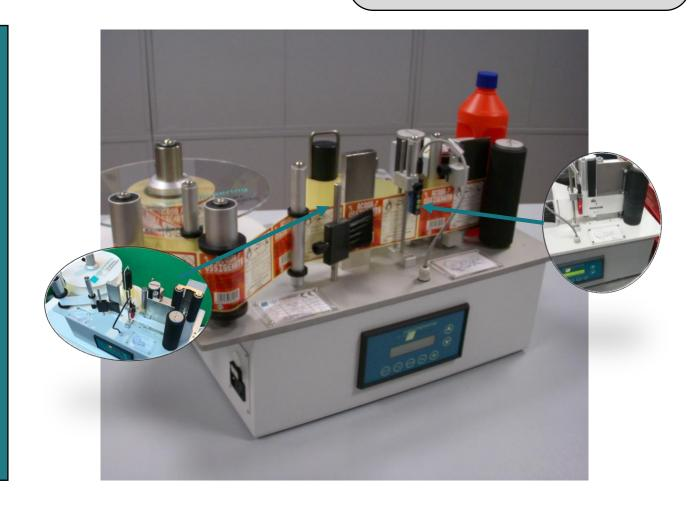
APPLY LABEL PARTY is suitable for the application of self-adhesive labels, for small production batches, on bottles, jars and cylindrical containers.
