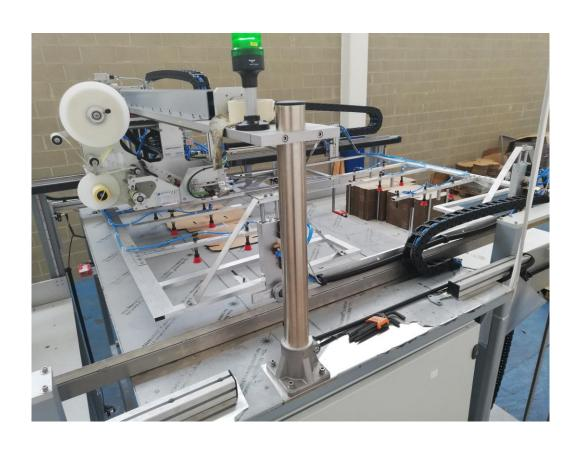
Flat carton handling system, complete with pneumatic labelling head suitable for the application of an identification label on the box, with its repositioning in the stacker device.
