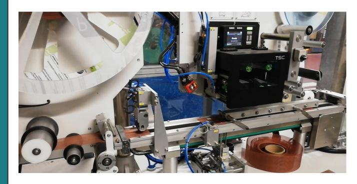
Print and Apply Head complete with cutting unit group and 4" print engine for the preparation of barcode label.
