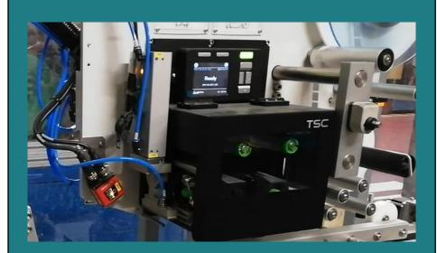
Print and Apply device mounted on a conveyor, complete with 4" printing group and cutting unit for tailor-made product preparation.
